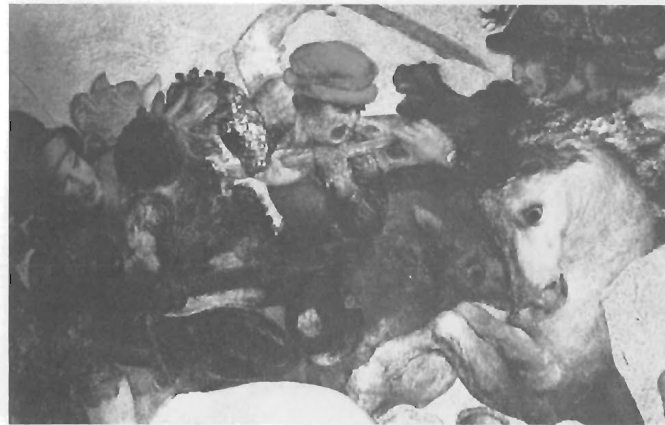
Here's how the ultrasonic probe system records a section of the Vasari painting on HP 1331A CRT display.
